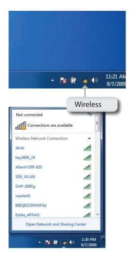
Highlight the wireless network (SSID) you would like to connect to and click the **Connect** button.
