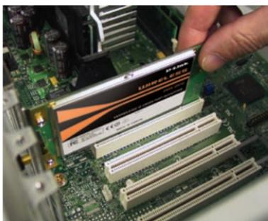
**Note:** Before installing, write down the serial number and hardware revision (e.g. A1) in case you need to contact technical support.
