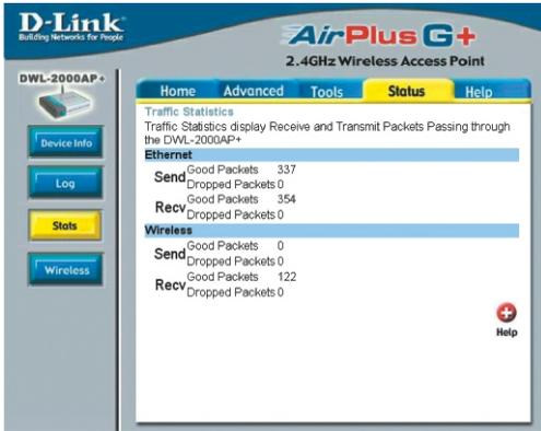
The screen above displays the Traffic Statistics. Here you can view the amount of packets that pass through the DWL-2000AP+. The traffic counter will reset if the device is rebooted.
