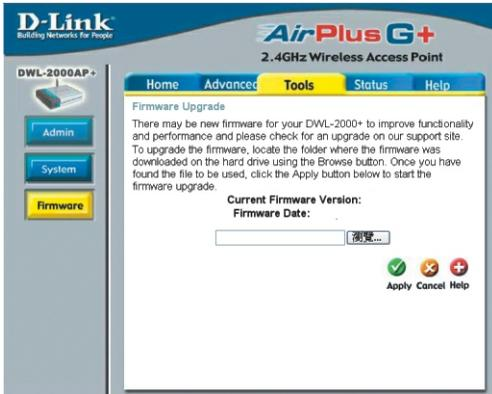
You can upgrade the firmware of the Access Point here. Make sure the firmware you want to use is on the local hard drive of the computer. Click on **Browse** to browse the local hard drive and locate the firmware to be used for the update. Please check the D-Link support site for firmware updates at <http://support.dlink.com>. You can download firmware upgrades to your hard drive from the D-Link support site.
