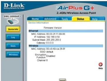
This page displays the current information about the DWL-2000AP+, such as the assigned IP Address and the wireless settings.
