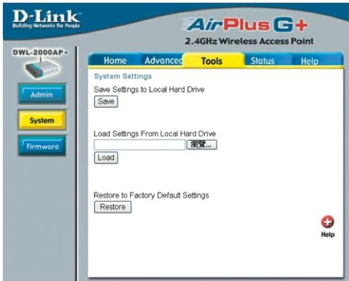
The current system settings can be saved as a file onto the local hard drive. The saved file or any other saved setting file can be loaded back on the DWL-2000AP+. To reload a system settings file, click on **Browse** to browse the local hard drive and locate the system file to be used. You may also reset the *Wireless Access Point* back to factory settings by clicking on **Restore**.
