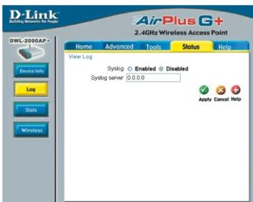
When you click on **Log Settings** in the previous window, the window at left appears. Select **Enabled** to save the log. In the **Syslog Server** field, input the IP Address of the computer on the network to which you wish to save the log settings. Click **Apply** to save the changes.
