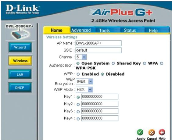
**SSID-** Service Set Identifier (SSID) is the name designated for a specific wireless local area network (WLAN). The SSID's factory default setting is **default**. The SSID can be easily changed to connect to an existing wireless network or to establish a new wireless network.
