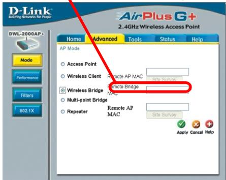
When using the DWL-2000AP+ in **Wireless Bridge** mode, you will enter the MAC address of the Remote Bridge.
