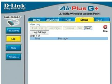
The Log keeps a running log of events and activities occurring on the Access Point. If the device is rebooted, the logs are automatically cleared. You may save the log files under Log Settings.
