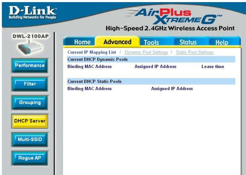
This screen displays information about the current DHCP dynamic and static IP address pools. This information is available when you enable the DHCP function of the DWL-2100AP and assign dynamic and static IP address pools.
