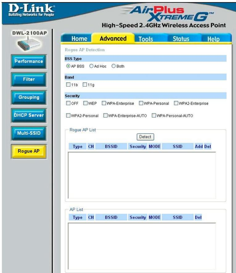
**BSS Type-** The Basic Service Set Type allows you to select from **AP BSS**, **Ad Hoc**, or **Both**.
