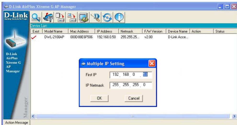
Select the AP that you want to assign an IP address to and click the IP button. Enter the IP address and IP netmask for the selected device and click OK.
