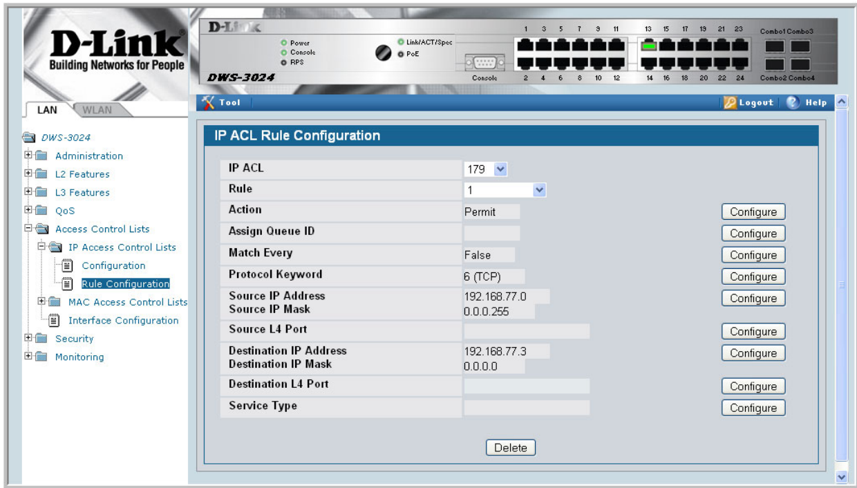
Figure 58. IP ACL Rule Configuration Page - Rule with Protocol and Source IP Configuration
