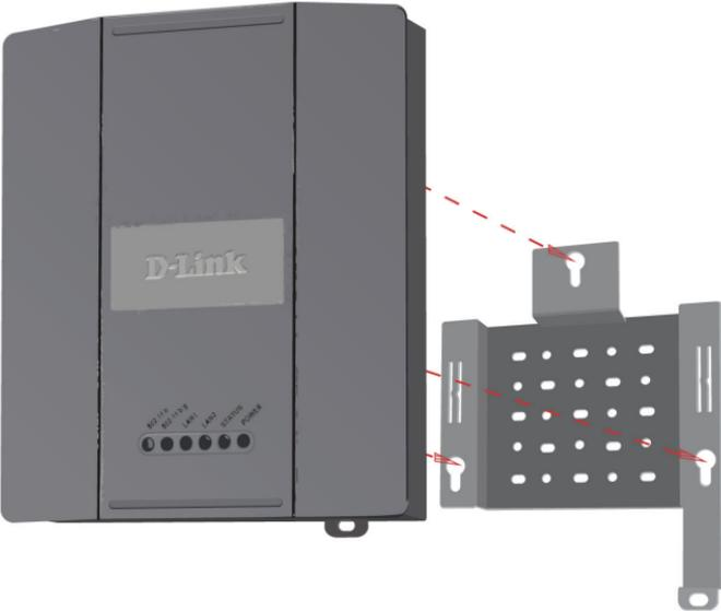
Step 5: Slide the DWL-8200AP down into the grooves on the mounting plate to secure it to the plate.
