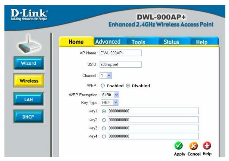
For this example we will be using the main AP configured with the settings below: (shown above in picture)
