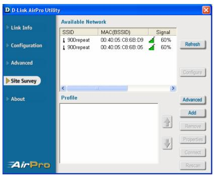
The reason that you see two wireless networks with the same SSID is because we have the main DWL-900AP+ #1 and also the DWL-900AP+ #2 as the repeater, which is retransmitting the signal with the same SSID.
