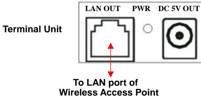
Finally, insert one end of the DC 5V Power Cable that is provided into the Terminal Unit, and the other end into the DC 5V/1A of the Wireless Access Point. The green LED of the Terminal Unit should light up.
