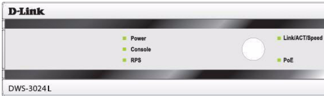
Figure 14: LED Indicators on DWS-3024L
