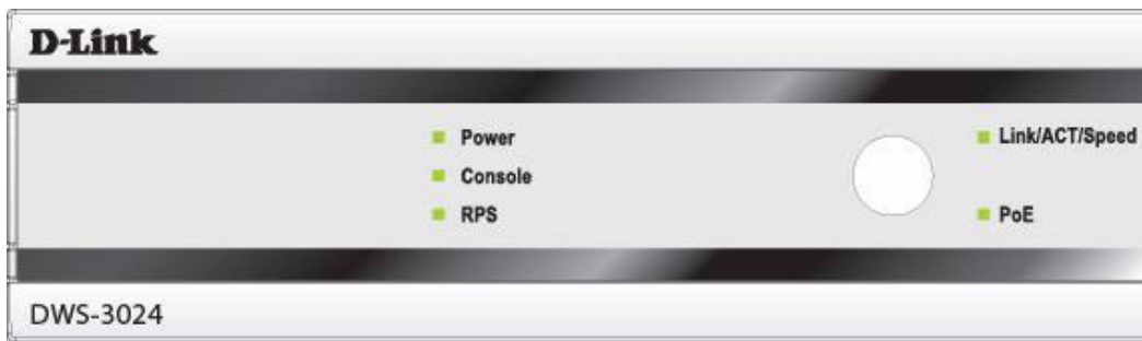
Figure 15: LED Indicators on DWS-3024
