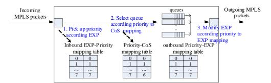
Once MPLS packets is received, if there is an inbound EXP to priority mapping entry for the FEC, the device will assign priority according to the inbound EXP. Otherwise, the priority is assigned according to 802.1p.
