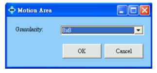
Configure the square size of software motion detection unit; this could be 4x4, 8x8, 16x16, or 32x32 in square. In 4x4 setting, you will have a larger area in motion detection, and vice versa.
