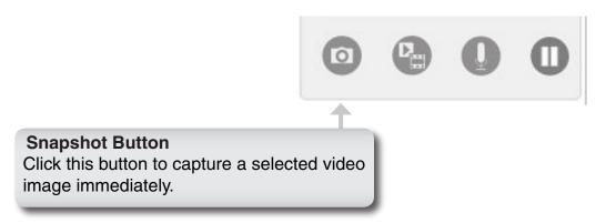
When a camera is selected and live video image can be seen in the main display or preview area, you can take a snapshot using the snapshot button. When this button is pressed, the system will show a dialogue window with the snapshot image and options as shown below:
