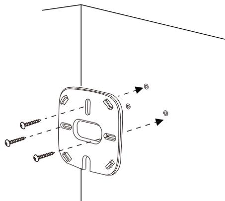
Figure 7: Securing the Mounting Plate
