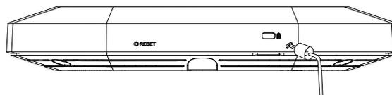
Figure 9: Inserting a Physical Lock
