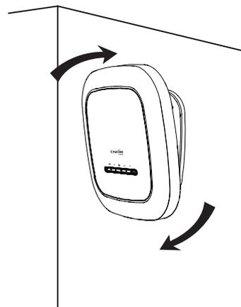
Figure 8: Placing The Access Point
