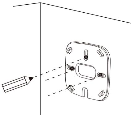
Figure 5: Mounting Panel Marking
