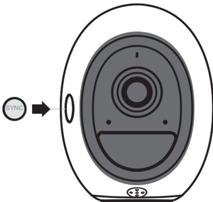
Once the hub has powered up, press the SYNC button on each camera to power them on.
