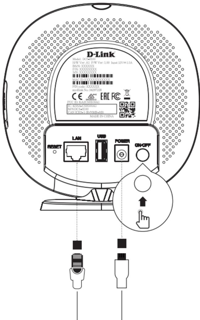
Plug the supplied Ethernet cable from your router or gateway into the port marked 'LAN'.
