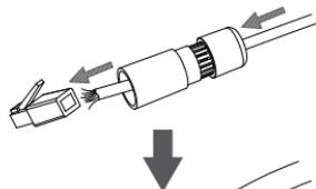
Crimp an RJ-45 connector onto the end of the cable.
