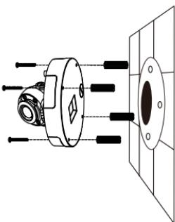
If you are mounting the camera to the ceiling, use a flathead screwdriver to remove the plastic hole cover from the bottom of the base, then guide the cables through the bottom.
