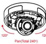
**Note:** The camera has a limited range of motion; if it stops when you are adjusting it, do not attempt to rotate or tilt the camera any further in that direction.
