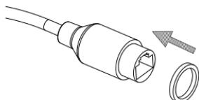
Thread bare Ethernet cable through the waterproof connector as shown.
