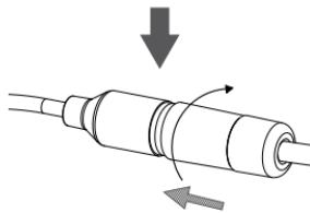
Screw the back part of the waterproof connector clockwise until there is a tight seal around the Ethernet cable.
