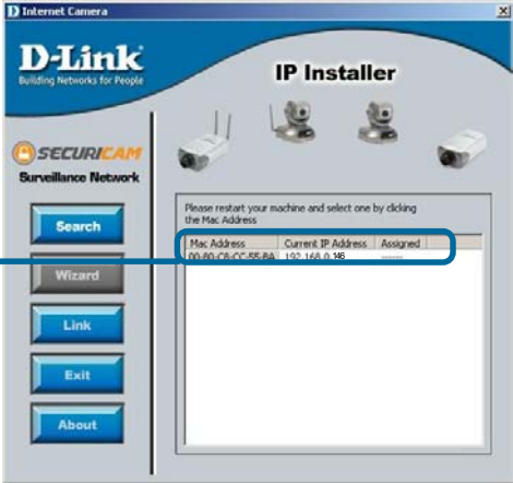
Assign a Local IP Address with IP Installer
