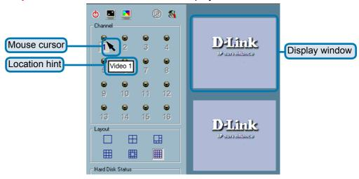
**Step 2:** Press and hold the left mouse button, and then move the cursor to a display window in the video area, which is shown below. Note that the cursor will change according to the area in order to indicate whether the area is droppable or not.
