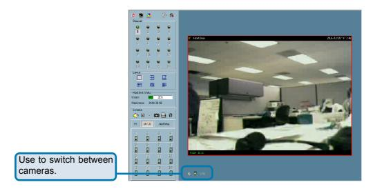
To view an individual camera from the multi-camera layout, double-click on the desired display window. You will see that the size of the display window is the same as the one-channel layout. Clicking the "Back" button in the upperleft corner of the video area will switch to the previous selected multi-camera layout.
