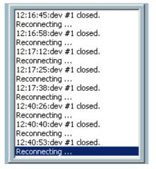
If you have checked the box for "Enable Motion Detect" or "Enable Digital Input" on "Camera Configurations > Alert Settings" screen, the alert message will show in the window shown above. Once the alert, caused by motion detection or a digital input level changer, is triggered, the alert message will be shown in this window. If there are more events than this window can display, a scroll bar will appear.
