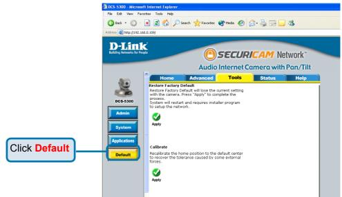
Click **Apply** on the screen to restore factory default settings. This means **any** changes made will be lost and the system will be reset to the initial status when shipped from the factory. After confirmation, the system will restart and require the **Installation Wizard** software program to locate the IP address of the **DCS-5300**.
