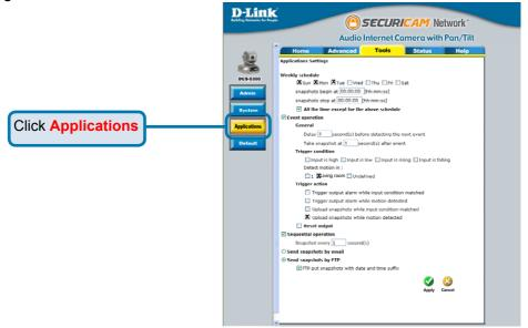
In this window, follow the steps below to set the application settings for snapshots to be recorded to an FTP site:
