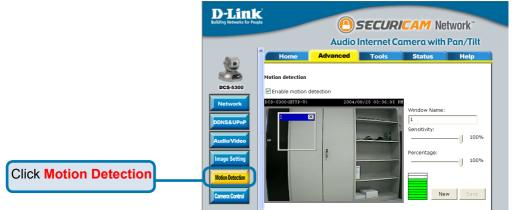
In this window, follow the steps below to ensure that motion detection is correctly enabled:
