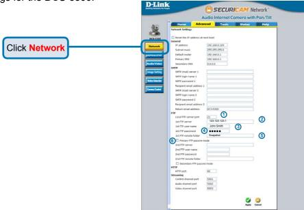
In this window, enter the settings for the FTP server you wish to record to. Optionally, you can enter settings for a secondary backup FTP server.
