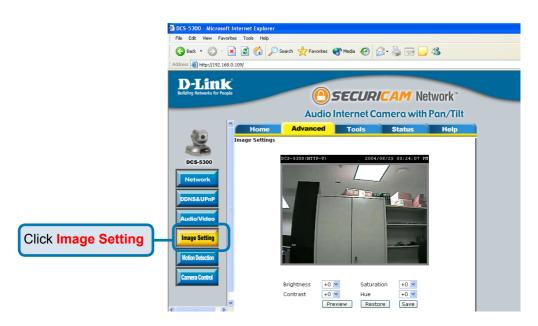
Click the Image Setting button from the Configuration screen to access additional settings that affect how the video image appears.
