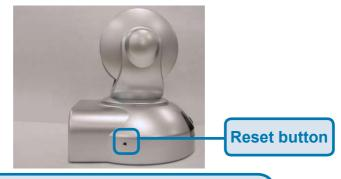
Restoring the factory defaults will result in the loss of any previous settings and will require running the Installation Wizard to return the **DCS-5300** to a normal state.
