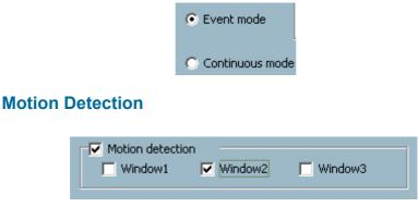
As shown above, you can check the windows to determine which window(s) will be used to trigger the recording. The motion windows are labeled in the order in which they are added when configuring motion detection for the camera. For example, Window1 is the first window added, regardless of if the name of the window has been changed.
