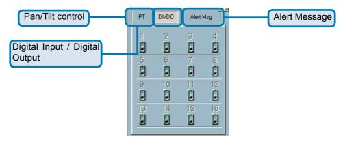
IP surveillance includes pan/tilt control, DI/DO (Digital Input / Digital Output) control, and an alert message receiver. Each of these are described in detail below
