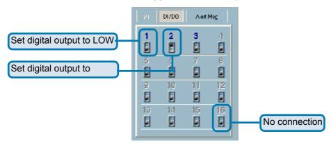
When the color of a DI/DO number is gray, that means the video has not yet been connected to a camera.
