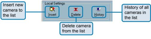
**Insert** – To insert a remote network camera to the camera list. Click the "Insert" button, an "Insert New Channel" dialog will popup, as shown below. Specify the IP address, port, and admin password of the network camera, click the "OK" button to close the dialog. Then the system will try to connect to the selected camera. If the connection succeeds, the camera will be inserted to the camera selection list.
