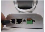
When you have a proper connection, the LED will turn from red to green. If you are directly connected to the camera via a crossover cable, the light may cycle on and off and your computer may show an intermittent loss of connectivity. This is normal until you have configured your Internet Camera.
