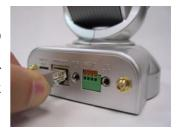
If you are connecting the **DCS-5300G** to a **802.11g wireless** Ethernet network, attach the two wireless antennas to the antenna connectors on the back panel of the **DCS-5300G**.
