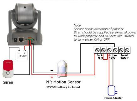
The above diagram shows a typical wiring configuration for a normally closed PIR motion sensor. Please refer to your specific motion sensor for the power supply connection to the device since this will be critical to the success of your installation. Note that the positive from the PIR is connected to the D- of the I/O port of the camera and the negative from the PIR is connected to the D+ of the camera I/O port.
