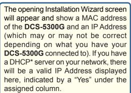
\*A DHCP server is a device that supplies IP Addresses to its clients that are on the same network.
