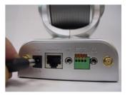
When you have a proper connection, the LED will turn from **red** to **green**. The light may cycle on and off and your computer may show an intermittent loss of connectivity, this is normal until you have configured your Internet Camera.
