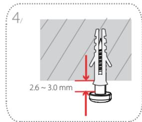
Twist the screws into the anchors, leaving the tops of the screws exposed from the surface. Do not over tighten the screws.
