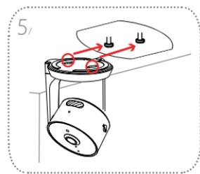
Align the mounting holes on the bottom of the camera with the screws. Slide the camera down to lock it into place.
