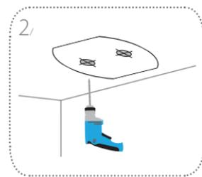
Use a 6 mm drill bit to drill two 3 mm deep holes as indicated on the alignment sticker.
