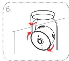
Twist the camera to your desired position. Go to the settings in the app and enable **Invert Image** if the image is up-side-down.
