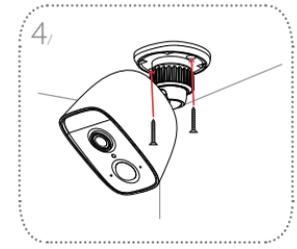
Align the camera mount's holes over the plastic anchors. Drive the screws into the anchors to secure the camera.
