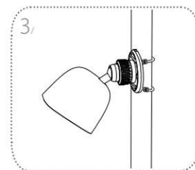
Fasten the plastic mounting ties around the pole to secure the camera.
