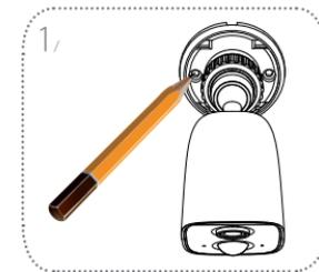
Place the camera against the wall where you want it to be positioned. Use a pencil to make two marks where the holes are located.
