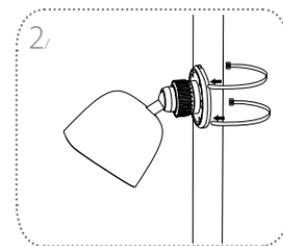
Thread the plastic mounting ties through the slots on the base of the device. Face the rough side of the plastic mounting ties to the pole to avoid slippage.
