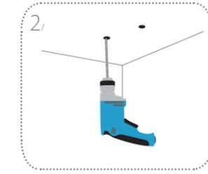
Use a 6 mm drill bit to drill two 26 mm deep holes over the pencil marks.
