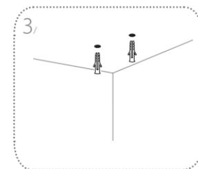
Hammer in the plastic wall anchors to support the screws.
