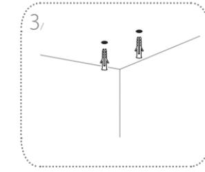
Hammer in the plastic wall anchors to support the screws.
