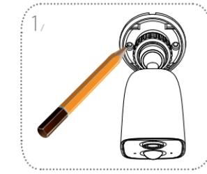
Place the camera against the wall where you want it to be positioned. Use a pencil to make two marks where the holes are located.
