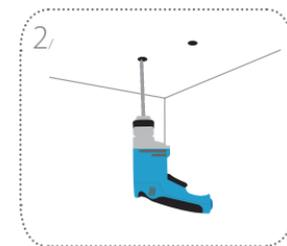
Use a 6 mm drill bit to drill two 26 mm deep holes over the pencil marks.
