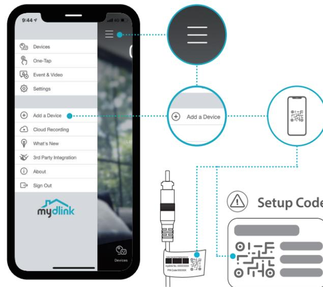
Tap the menu button ☰ then tap **Add a Device**. Scan the Setup Code on the device or on the **Setup Code** page of this Quick Installation Guide, then follow the app instructions.
