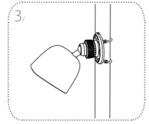
Fasten the plastic mounting ties around the pole to secure the camera.
