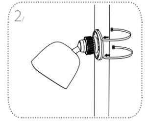
Thread the plastic mounting ties through the slots on the base of the device. Face the rough side of the plastic mounting ties to the pole to avoid slippage.
