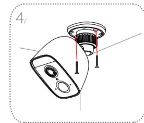
Align the camera mount's holes over the plastic anchors. Drive the screws into the anchors to secure the camera.
