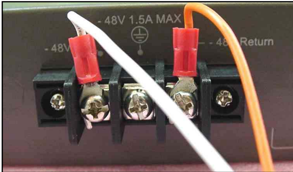
Figure 2- 4. Power connections attached to contacts on assembly
