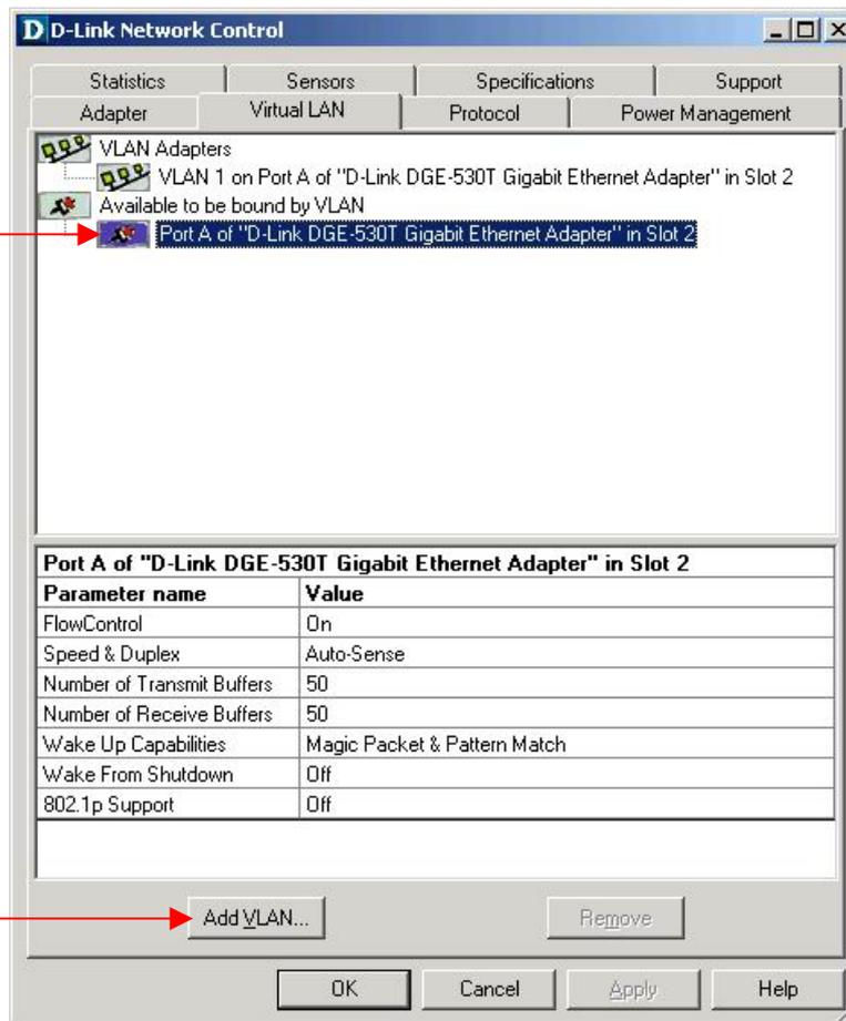
To add a VLAN setting to this window, click the **Add VLAN** button at the bottom of this screen, which will open the following configuration window.
