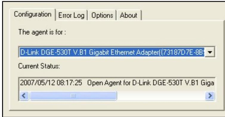
The Configuration Tab has two fields. The first field, “**The agent is for:**”, allows the user to choose an Ethernet card to configure, from a pull down menu. The “**Current Status**” is a read only field which displays the most recent action made by the Ethernet card.
