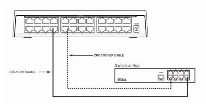
Switch connected to a port on a hub or switch using either a straight or crossover cableany standard Ethernet cable is fine
