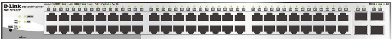
Figure 1.13 – DGS-1210-52P Front Panel
