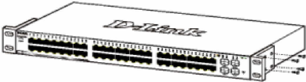
Figure 2 – Attach the mounting brackets to the Switch
