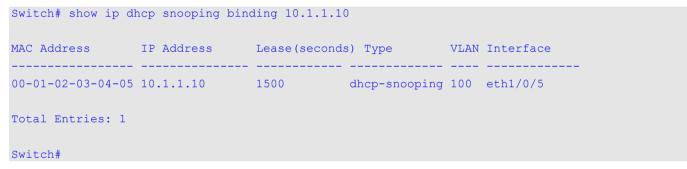
This example shows how to display DHCP snooping binding entries by IP 10.1.1.10 and MAC 00-01-02-00-00-05. Switch# show ip dhcp snooping binding 10.1.1.10 00-01-02-03-04-05
