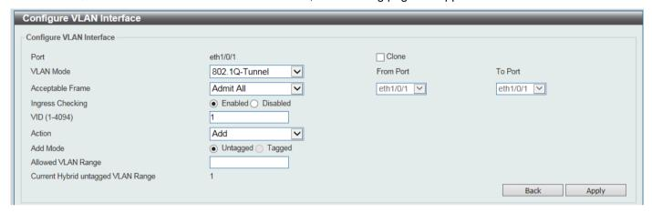
Figure 5-24 VLAN Interface (802.1Q-Tunnel) Window
