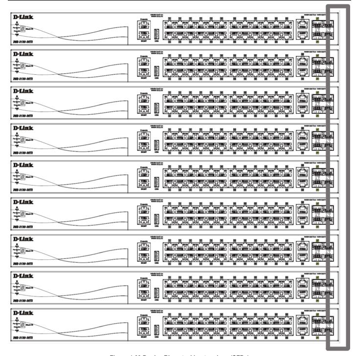
Figure 4-69 Duplex Ring stacking topology (SFP+)
