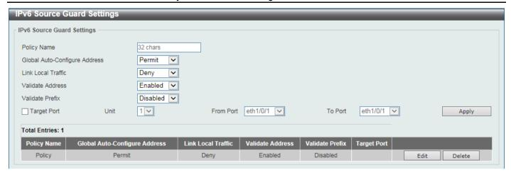
Figure 9-615 IPv6 Source Guard Settings Window
