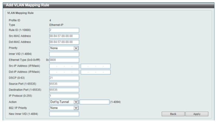
Figure 5-45 VLAN Mapping Profile (Ethernet-IP, Add Rule) Window
