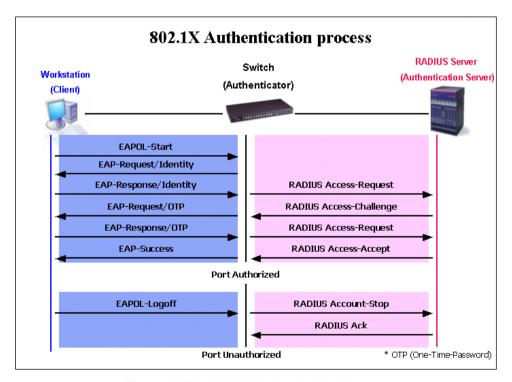
Figure 9-9 The 802.1X Authentication Process
