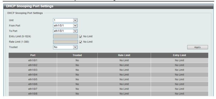
Figure 9-40 DHCP Snooping Port Settings Window
