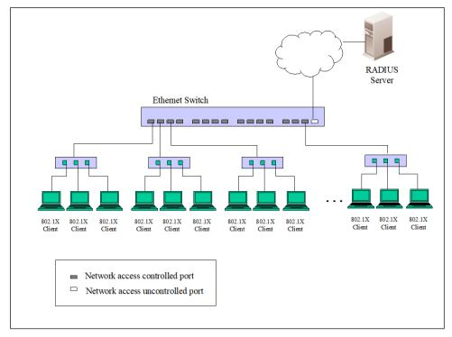
Figure 9-11 Example of Typical Host-based Configuration
