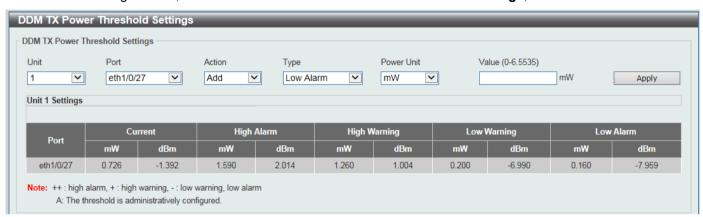
Figure 10-271 DDM TX Power Threshold Settings Window
