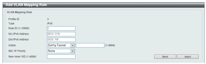
Figure 5-44 VLAN Mapping Profile (IPv6, Add Rule) Window
