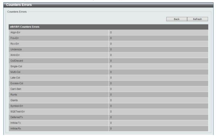
Figure 11-10 Interface Counters (Show Errors) Window
