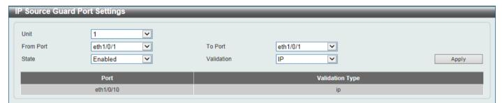
Figure 9-51 IP Source Guard Port Settings Window
