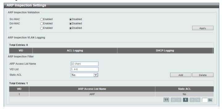
Figure 9-46 ARP Inspection Settings Window
