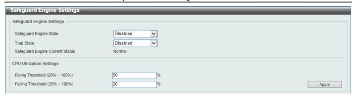
Figure 9-80 Safeguard Engine Settings Window
