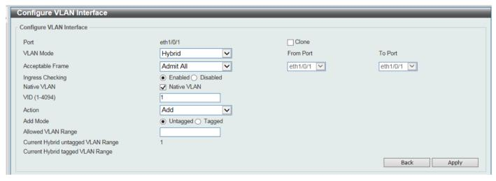
Figure 5-22 VLAN Interface (Hybrid) Window
