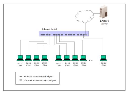
Figure 9-10 Example of Typical Port-based Configuration
