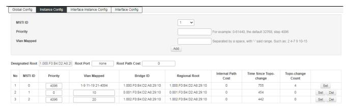
5) In the domain 12345678, configure the root bridge and backup root bridge of MSTI1 and MSTI2, configure switch A as the root bridge of MSTI2, and configure switch B as the backup root bridge of MSTI1. The operation steps are the same as 5, so I won't repeat them. After the above configuration, the network is pruned into a tree shape to achieve the purpose of eliminating loops.
