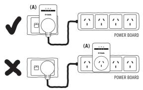
**DON'T** plug the Adaptor (A) directly into an extension cord, surge-protection board or powerboard.
