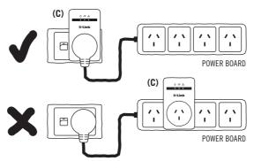
**DON'T** plug the Adaptor **(C)** directly into an extension cord, surge-protection board or powerboard.
