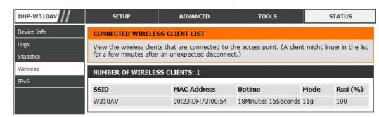
Mode: Shows the mode the device is using to connect to your DHP-W310AV. This should be 11b, 11g, or 11n.
