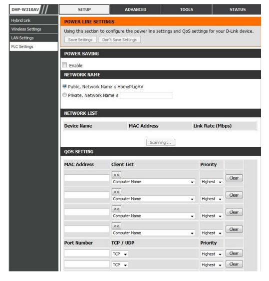
MAC Address/ Select a device from the Computer Name dropdown box and then click the << above Computer Name to automatically fill in Port Number: the device's MAC Address. Or, Set the priority for the device under the Priority dropdown box. Clear settings for a rule with the Clear button. Remember to click Save Settings after making changes.
