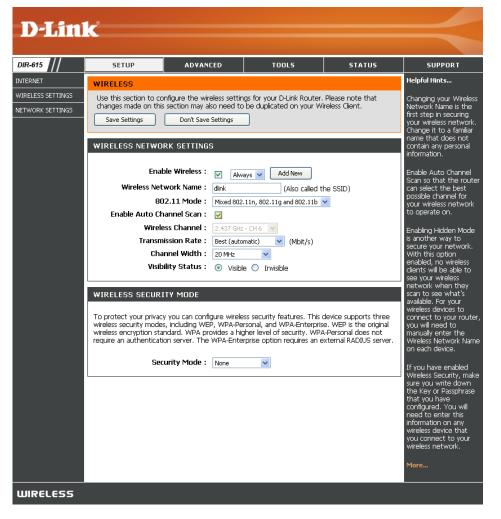
Wireless Channel: Indicates the channel setting for the DIR-615. By default the channel is set to 6. The Channel can be changed to fit the channel setting for an existing wireless network or to customize the wireless network. If you enable **Auto Channel Scan**, this option will be greyed out.
