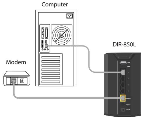
5. Reconnect the power adapter to your cable or DSL broadband modem and wait for two minutes.
