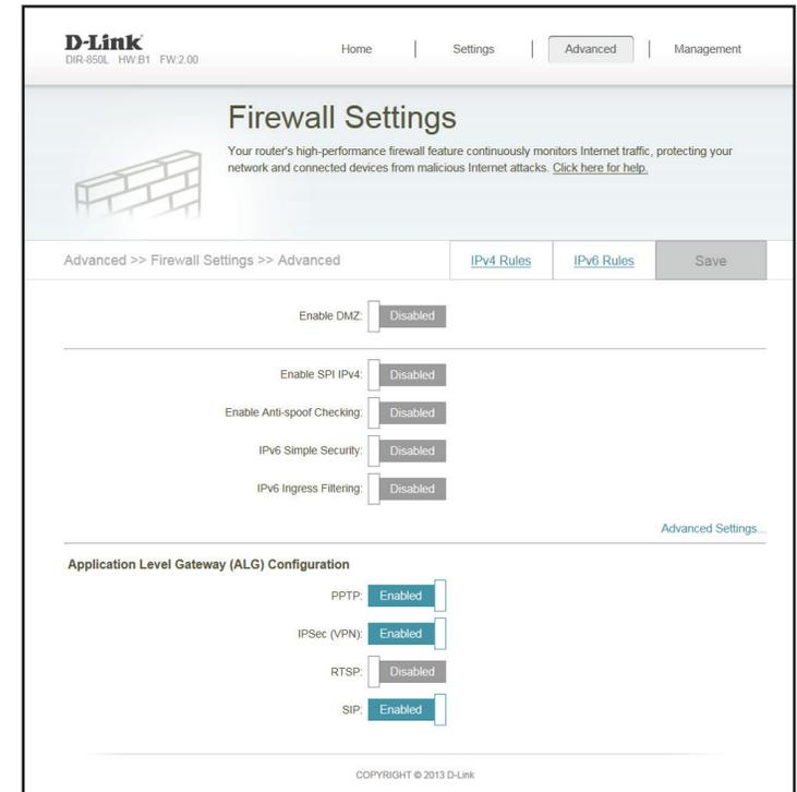
**IPSec (VPN):** Allows multiple VPN clients to connect to their corporate network using IPSec. Some VPN clients support traversal of IPSec through NAT. This Application Level Gateway (ALG) may interfere with the operation of such VPN clients. If you are having trouble connecting with your corporate network, try turning this ALG off. Please check with the system administrator of your corporate network whether your VPN client supports NAT traversal.
