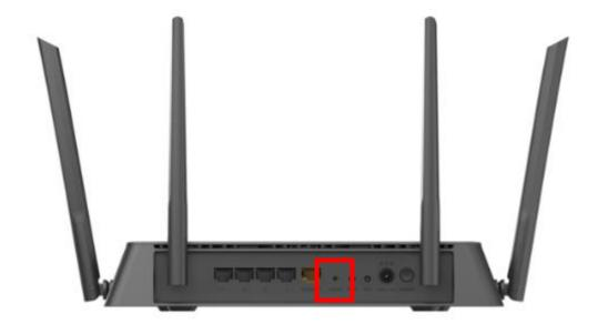
**Step 2:** The unit will reboot automatically. Once the power light stops blinking, the unit has been reset and is ready to use. **Resetting the router does not reset the firmware to the previous version, but it will change all settings back to factory defaults.**
