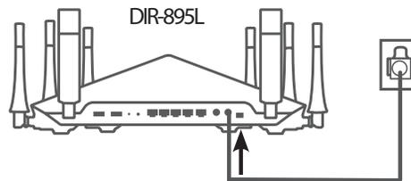
**Note:** Extending the network to your desired location via Ethernet may require the purchase of additional cable. Maximum CAT5e cable length is limited to 100 meters. Use a Gigabit-capable Ethernet connection where possible to ensure the best networking experience. This unit is to be used with power supply model DA-60N12.
