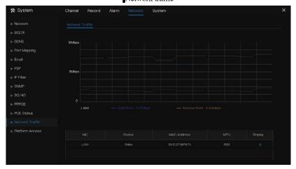
There are two rates, transmit rate and receive rate. The status of LAN(s) show on list.
