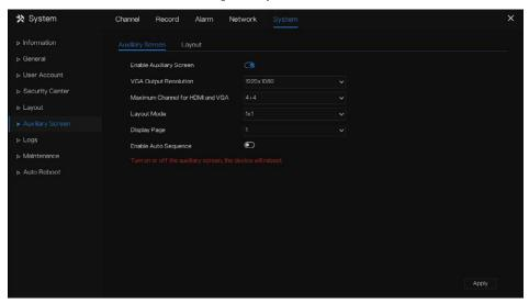
Step 3 Set the Output Resolution, Decoding Ability(main + auxiliary), Layout Mode, Display Channel.
