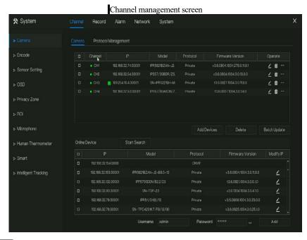
: Modify device parameters, remote channel is based on cameras (human body temperature has two remote channels, fisheye cameras have four remote channels) as shown in Figure 7-2.
