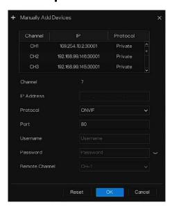
Step 2 Input IP address, port, user name and password of this camera. Double click the online camera IP to copy its configuration. Quick change of other channel's parameters can be done. Step 3 Select a protocol from the drop-down list(ONVIF, Private, custom protocols). Remote channel is only used for multi channels cameras, such as human temperature cameras, fisheye cameras, and so on.
