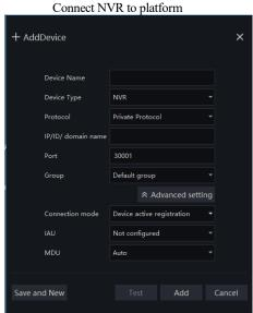
3: the CMU, MDU and IAU servers of platform should be mapped to the ports to external network in advance.
