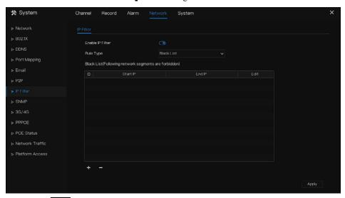
Step 2 Click next to **IP Filter** to enable the function of IP Filter.
