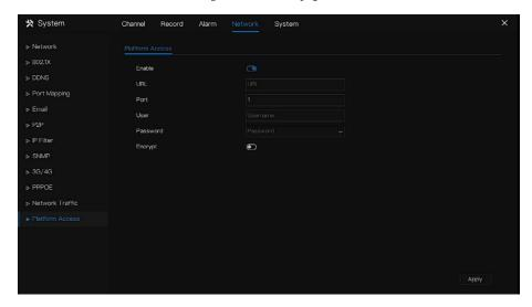
Step 2 Input the parameters. The URL and port are the platform server IP address and port Step 3 The name and port are the platform's login name and password.
