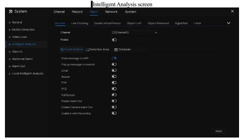
Step 2 Select one action to set the alarm.(Intrusion, Line crossing, Single virtual fence, Double virtual fences, Object left, Object removed, Signal bad, Loiter, Multi loiter, Abnormal speed, Converse, Illegal parking, Personnel count, Fence, Enter area, Leave area, Advanced).
