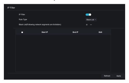
Step 2 Click **Enable** to enable the IP filter function.
