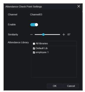
Step 3 Enable the function, set similarity and tick the library, all face detection cameras can be set the check points.
