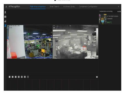
If users enable the mask detection, the snapshot results will reminder wear mask or no mask.
