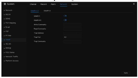
Step 2 Click next to **SNMPV 1** to enable the function . The interface is shown as Figure 7-67.
