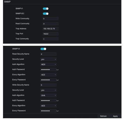
Step 2 Input the information of SNMP (simple network management protocol). there are three types of that function. Users can apply that if need.
