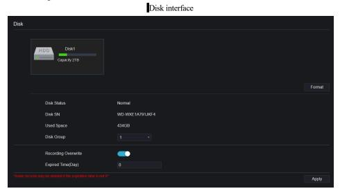
Step 2 You can view the information like capacity, disk status, disk SN code and used space.
