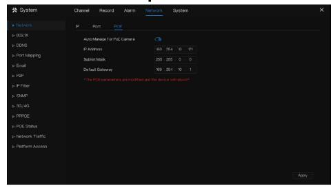
Step 2 The NVR will deploy IP addresses to the cameras connected to POE immediately.
