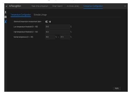
At temperature comparison interface, users can set low temperature threshold, high temperature threshold, and normal temperature.
