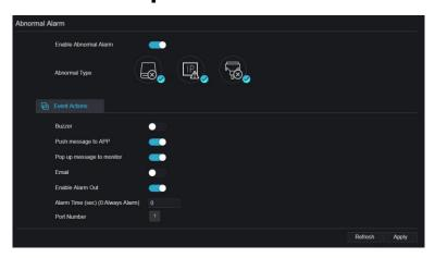
Step 2 Enable the button, tick alarm type.
