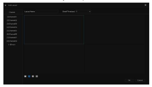
Step 3 Input the layout name, select dwell time from the **SEQ** Dwell time drop-down list(the display screen will loop play the real time video according to setting time).
