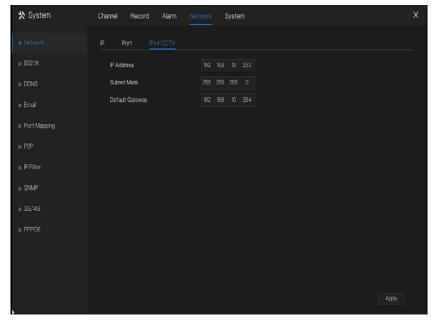
Step 2 Input the IP address, subnet mask, default gateway.
