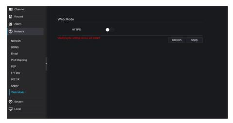
Step 2 Enable the https, the device will restart and start https secure.
