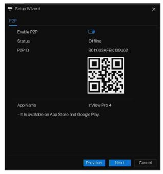
Step 8 Enable the P2P, user can use mobile devices to manage the NVR by scanning the P2P ID, if the mobile phone has loaded the InView Pro 4(search the APP at App Store or Google Play).
