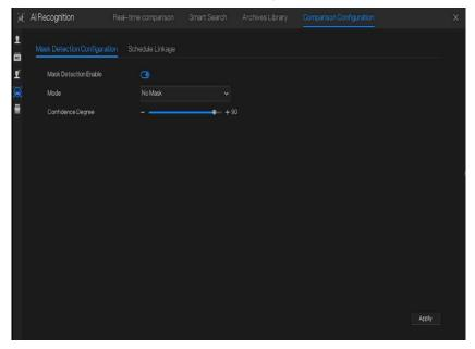
Enable mask detection, choose the mode (with or without a mask). Set the confidence degree, the default value is 90.
