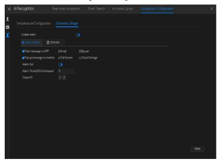
Enable alarm, set the schedule linkage, it will send alarm information if the temperature is higher than low threshold and lower the normal temperature, or higher than normal temperature and lower than high threshold.
