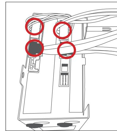
5. Re-attach the drive bay bracket to the device enclosure by sliding the tabs into the holes and using the screws provided to secure it.
