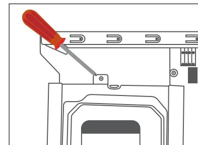
6. Re-attach the top cover by sliding it over the device. Re-insert the screw in rear of the cover to secure it.
