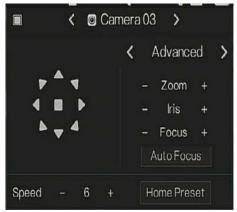
Figure 6-8 PTZ adjust screen
