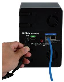
**Step 5 -** Connect the power adapter to the power receptacle.
