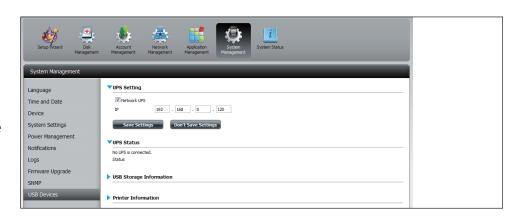
If a UPS device is connected to the USB port on your NAS, you can select either Stand-Alone or Master mode. If you select Master mode, you will have to enter the IP address(es) of the network UPS slaves to notify them in the event of a power failure. For more details, refer to the **UPS Connectivity** section.
