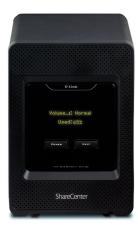
This displays the drive name and usable storage capacity.
