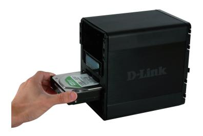
**Step 2** - Insert up to four 3.5" SATA hard drives into the drive bays.
