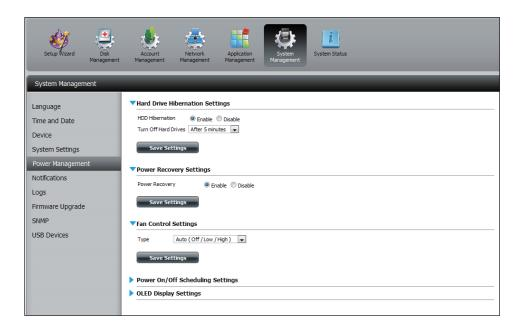
You can control the speed of the fan using three different settings and you can power off the device at scheduled times for each day of the week.
