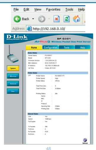
At the **Configuration** window, write down the **Port Name** for future reference. You will need this information later in the configuration process. The **Port Name** shown here is only an example.
