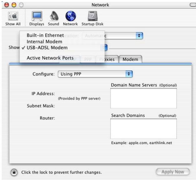
4. Select the **Modem** tab. In the **Modem** pull down menu, select **ADSL USB Modem**. Uncheck **Wait for dial tone**
