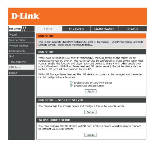
To setup Printer Server, press **setup** button in **USB SETUP** window enter the server configuration page
