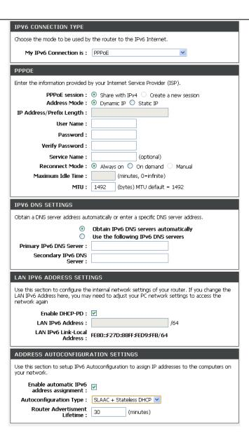
**SLAAC+RDNSS** to set computers on Router network obtained IPv6 address by RDNSS
