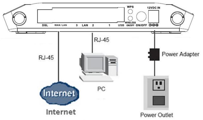
Figure 4 Ethernet uplink connection
