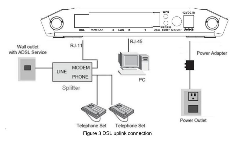
**Step 1** Connect the **DSL** port of the router and the Modem port of the splitter through a telephone cable; connect the phone to the phone port of the splitter through a telephone cable; and connect the Line port of the splitter to the uplink telephone jack on the wall.
