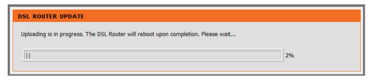
After finishing the upgrade your modem router will restart automatically and you will be prompted to relogin. You can verify the firmware version in the top right corner of the screen.
