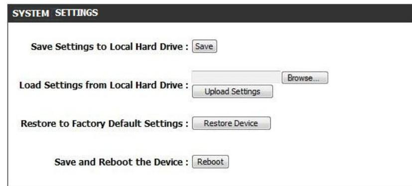
on this router. To reset the router to its factory default settings, click the **Restore Device** button of **Restore to Factory Default Settings**. You will be prompted to confirm your decision to reset the router. The router will reboot with the factory default settings.
