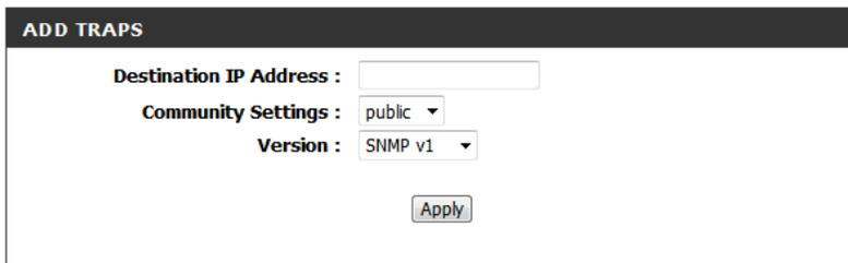
The screenshot shows the 'ADD TRAPS' configuration page. It includes three fields: 'Destination IP Address' with an empty text input field; 'Community Settings' with a dropdown menu showing 'public'; and 'Version' with a dropdown menu showing 'SNMP v1'. An 'Apply' button is located at the bottom right of the form.
