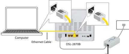
Plug the power adapter into your modem router and connect to an available power outlet.
