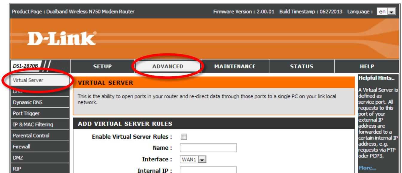
**Step 4.** Tick the **Enable Virtual Server Rules** option and enter the rule details. We are using opening port for Remote Desktop service as an example:
