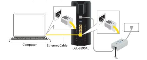
Plug the power adapter into your modem router and connect to an available
