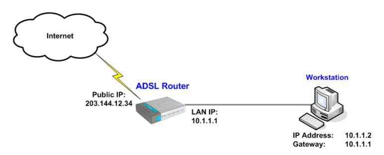
This example shows how to open port 3389 (which is used by Remote Desktop service) in the DSL-502T router running firmware version 2.00B02 or above. You need to find out what ports your application is using. For example WEB server (HTTP) is using port 80 TCP, PCAnywhere uses ports 5631 TCP and 5632 UDP, etc.
