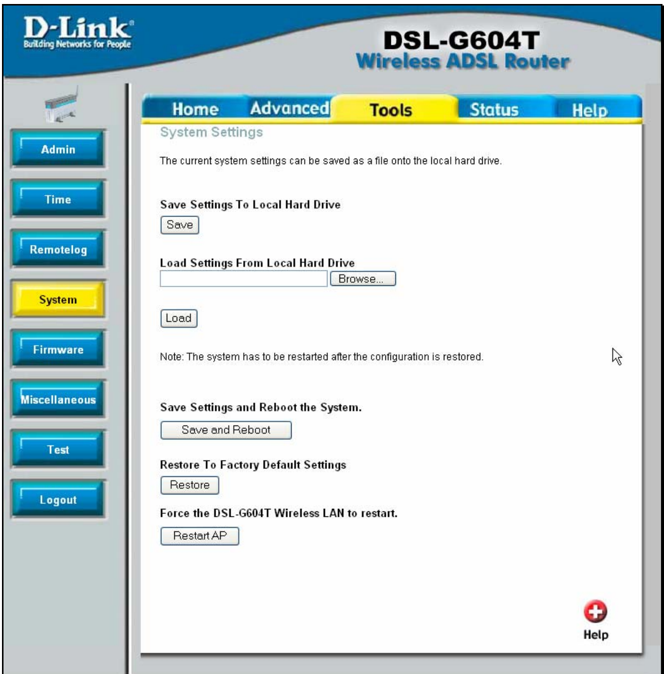
Figure 6- 4. System Settings window
