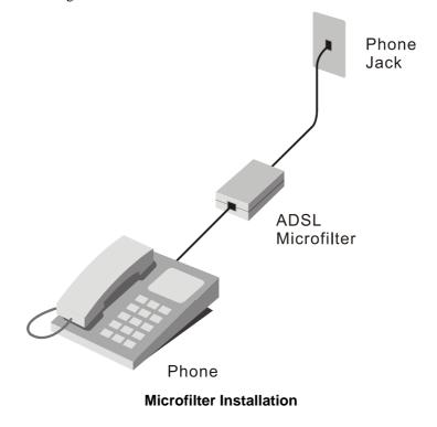
**Important:** Do not install the microfilter between the Router and the telephone jack. Microfilters are only intended for use with regular telephones, Fax machines and other regular telephone devices.
