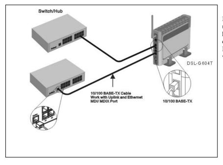
If you wish to reserve the uplink port on the switch or hub for another device, connect to any on the other MDI-X ports (1x, 2x, etc.) with a crossed cable.
